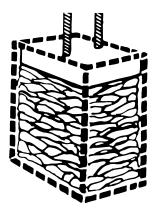
The trash in a full compactor bag will be about 1/4 the size of its original bulk.
